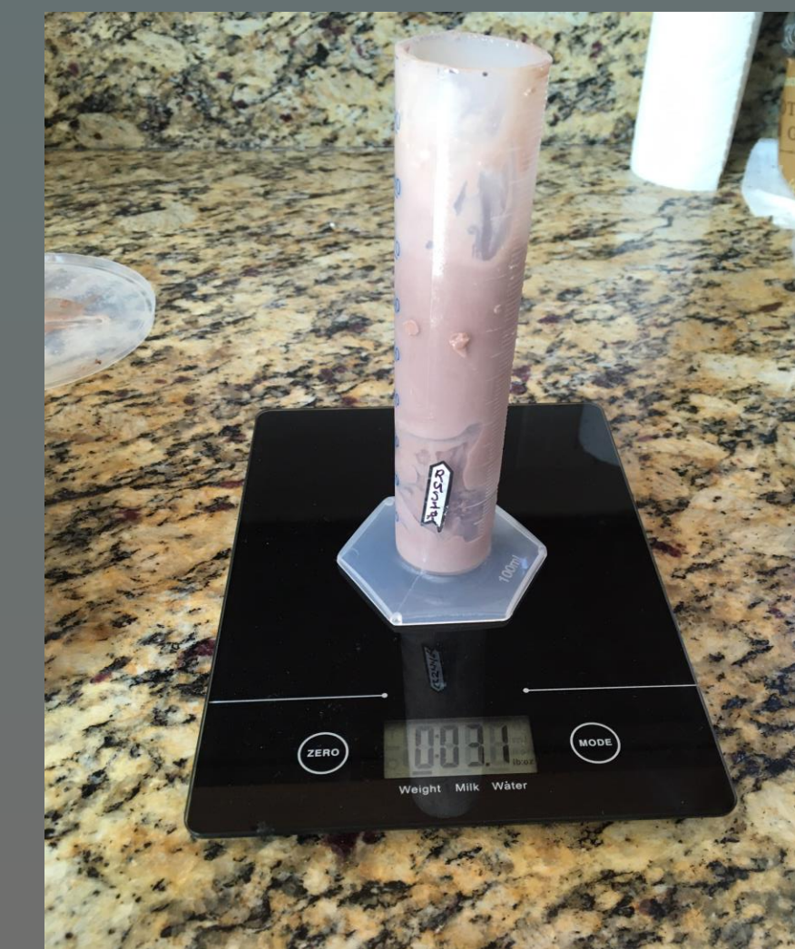
Measuring the Density of Ice Cream
